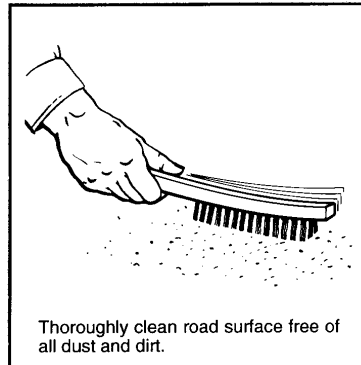
Figure 20: Step 1 – installation for retroreflective road pavement markers for hydrants.
