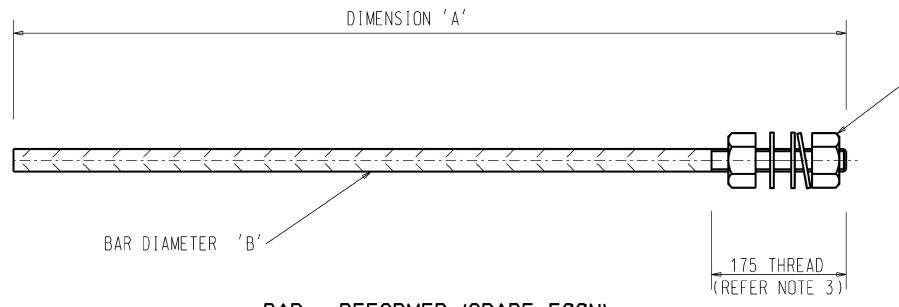
GALVANISED HEX NUTS (2) FLAT WASHERS (2) & SPRING WASHER (1) (TO BE SUPPLIED FITTED TO BOLT).
