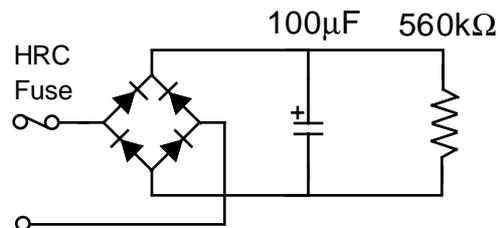
Figure B2 Inverter Load for Voltage Limit test to replace no load conditions.
