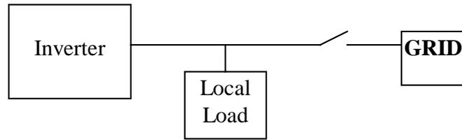
Figure B1 Circuit for Tests under actual grid trip conditions
