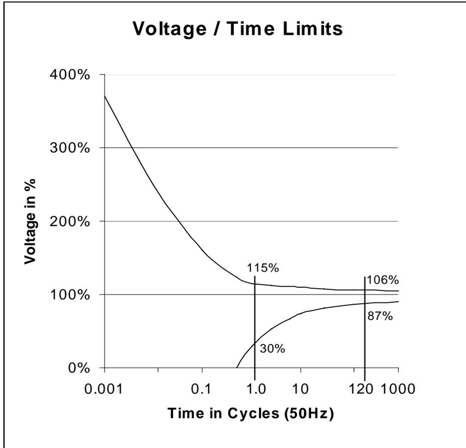
**Figure 1 Voltage/time limits. (Voltage must remain in area between curves.)
