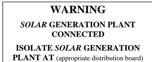
**6.1.1.2** *Main switchboard or distribution board where the inverter energy system is connected.*
