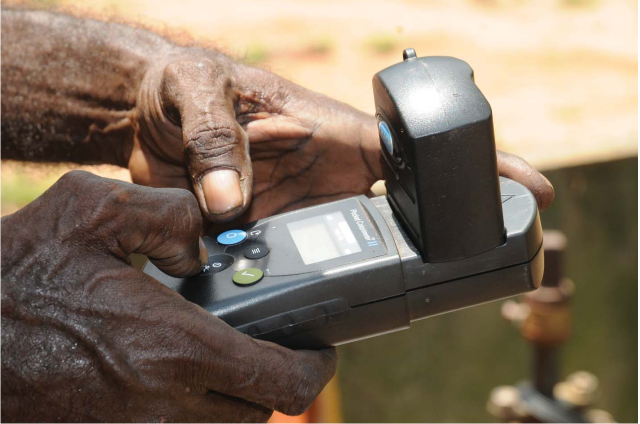
ABOVE > MEASURING CHLORINE RESIDUALS WITH A PORTABLE CHLORINE METER
