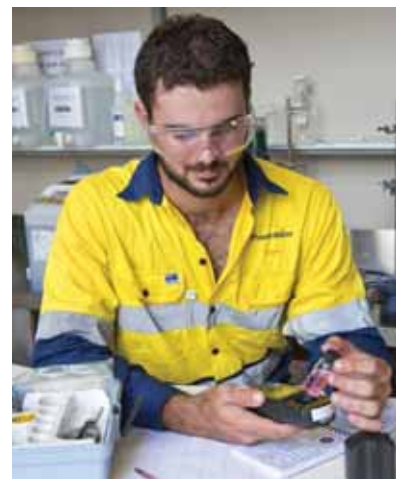
ABOVE ► WATER QUALITY TECHNICIAN JORDAN PHASEY CALIBRATING A CHLORIMETER
